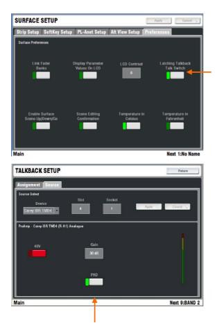
The lower part of the Source page provides access to the preamp settings and meter if a MIC/LINE input has been selected, or the digital trim and meter if a digital input has been selected. Use these to set the Talkback level.
